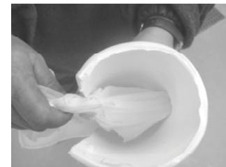
14) If TL-100 does not dislodge from the plastic- simply trim away nylon around the light. It is not vital that the light be removed during the final stages of finishing the orthosis.
